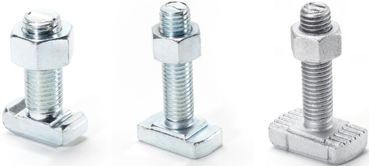
All JORDAHL® T-bolts are purpose made to ensure reliable and accurate connection with the range of JORDAHL® channels. The T-bolts face enter into the channel profiles and rotate 90 degrees to safely lock in position. Lines on the end of the T-bolts indicate the head position for easy checking after installation.
