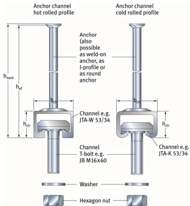
Figure 3.1: Anchor channels
