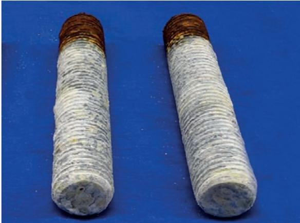
JACOB bar threads after 480 hours of salt spray test.
