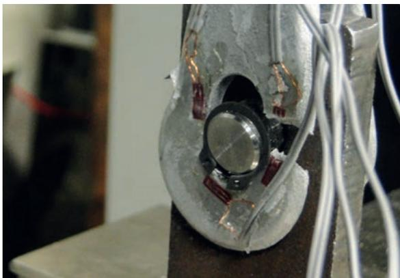
Tensile test on M16 fork using a break load of 150 kN.
